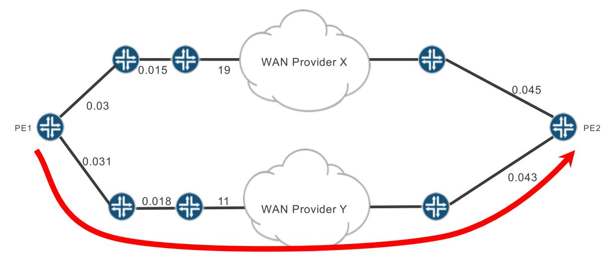
Link delay values are measured by routers and reported to Controller periodically. Red LSP carries delay-sensitive traffic so Controller uses delay as the cost function when computing the path.
