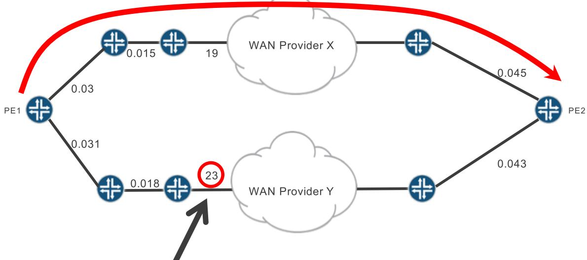
Step change in delay via Provider Y (due to reroute or protection event within Provider Y) Controller reroutes red LSP via Provider X.
