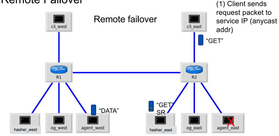
(2) OG add segment list and forward to remote OG cluster according to connection table(3) agent replies directly to client (DSR), using service IP as source addr
